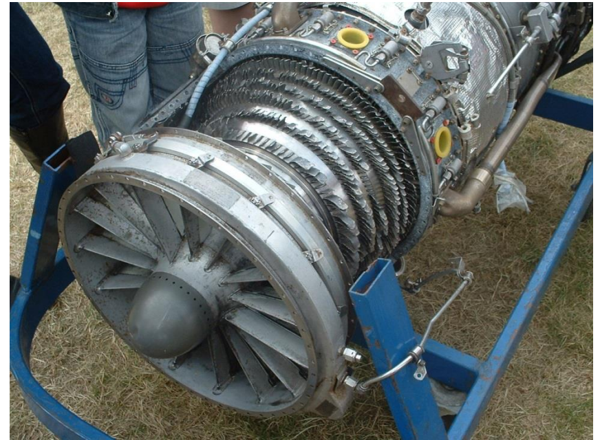
Inside of a jet engine after a bird strike / Wikimedia Commons
